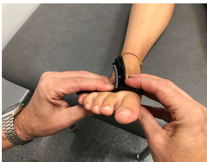
Figure 3. Quantifying first-ray dorsiflexion with the meter.
